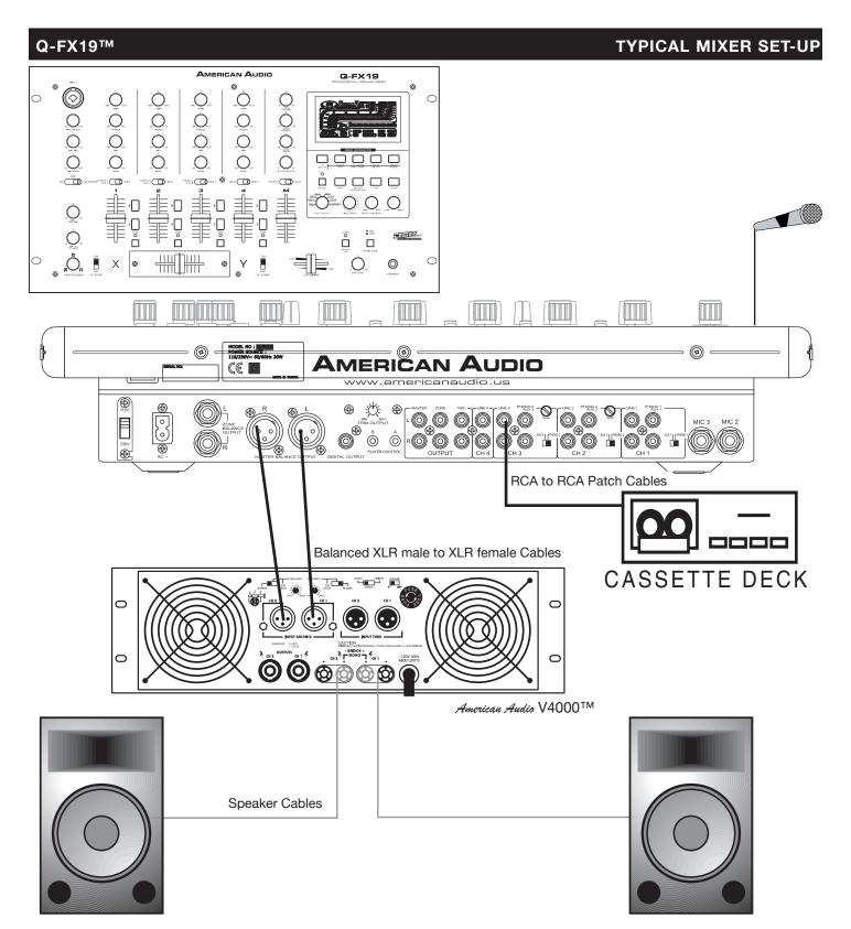
Typical Balanced Output Set-up
